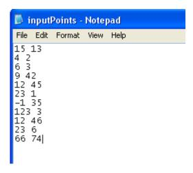
Where each line contains a set of numeric values (b, h). The value b is the base of the right triangle while the value h is the height of the right triangle.
