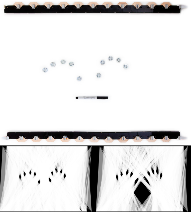
Figure 10: Two-Sided Sensing with ZeroTouch. The data from the sensor shown above is visualized both with the pen (right) and without (left). Notice the distorted shape that the pen leaves, compared to Figure 9.
