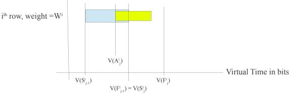
From the figure above, If the current packet j arrived when the previous packet j-1 was still being transmitted then the current packet will be started only after the previous packet has finished transmitting. In this case virtual start time of jth packet = virtual finish time of the j-1 packet.
