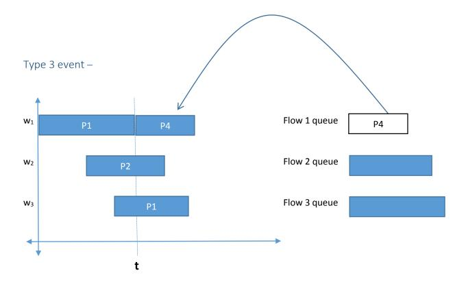
Packet P4 moves over from flow queue after P1 ends.
