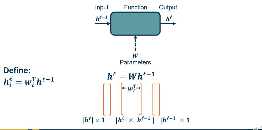
Fully Connected (FC) Layer: Forward Function
